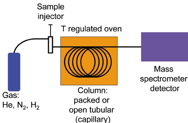
**Figure 1.4:** Processes involved in measuring metabolite abundance using GC-MS. The sample is first vapourised and then transferred to a chromatographic column. Compounds are separated in the column via their interaction with the column walls. Samples leaving the column are ionised and passed through a magnetic field which separates the ionised compounds based on their charge-to-mass ratio. [GC-MS schematic](#) was created by K. Murray and shared under [CC BY-SA 3.0](#).
