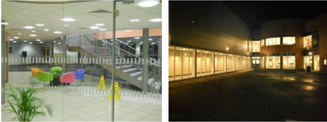
Figure 5.23. Internal lights ON in the entire circulation space in Building C outside core occupancy hours
