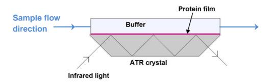
**Figure 7.3** Simplified depiction of an ATR-FTIR sample and infrared beam configuration, with the sample cell in flow-through mode.
