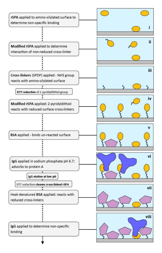
**Figure 7.4** Flow chart and cartoon diagrams to illustrate a procedure used to assess rSPA non-specific binding to silica, rSPA cross-linking, IgG adsorption and IgG non-specific binding. The surface was analysed by ATR-FTIR.
