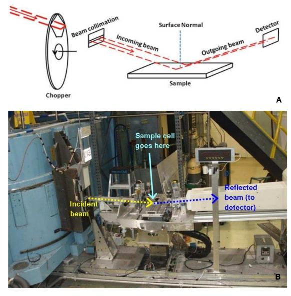
**Figure 6.1** (a) Schematic representation of a neutron reflectivity instrument showing a pulsed collimated beam of neutrons undergoing specular reflection from a sample surface. (b) Photograph of the NG7 reflectivity rig at the NIST Center for Neutron Research. The image illustrates the very low angles at which specular reflection occurs – dotted lines indicate the path of the neutron beam.
