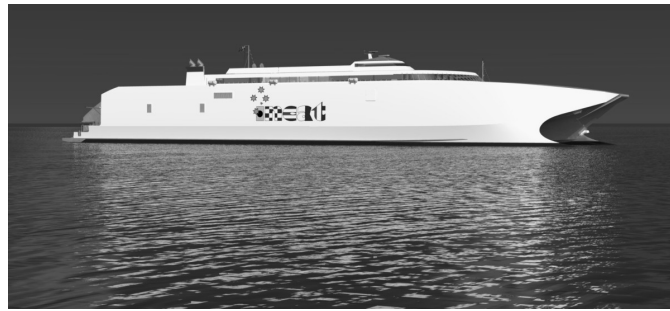
Figure 1: Proposed design of a 130 m medium-speed catamaran.
