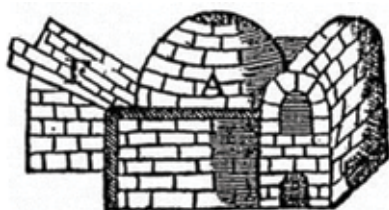
Fig. 6: 'Dragon furnace' for silver smelting in the Bolivian Andes (after Barba 1640).
