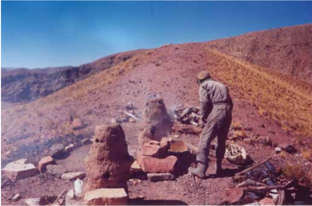
Fig. 2: A huayrachina smelting furnace in use for lead production near Porco, Bolivia (photo B. Mills).
