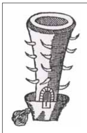
Fig. 1: A huayrachina silver-smelting furnace in the Bolivian Andes (after Barba 1640).
