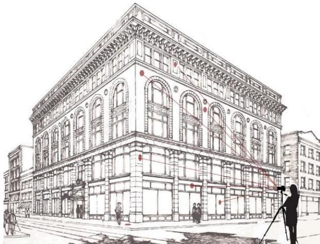
Figure 11. Illustration of the spot luminance measurements using a luminance meter on a tripod<sup>152</sup>.
