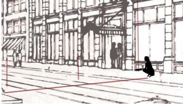
Figure 10. Illustration of the process of taking  $E_h$  measurements, using an illuminance meter at above 0.20 metres from the floor.
