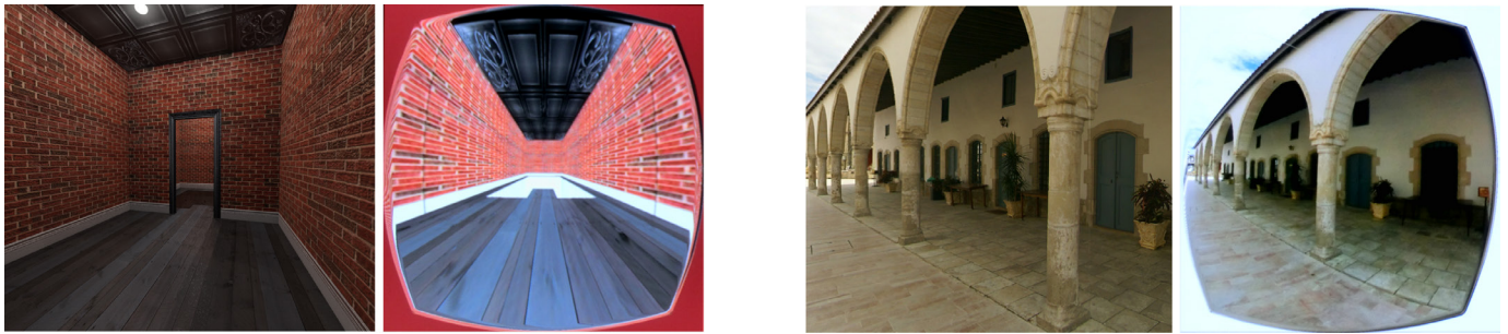
Fig. 2. Images of two virtual environments designed for the DFE frameless renderer, along with photos of the right eye region of the display showing them being drawn in real-time. The Pit Room (left) is a synthetic environment made up of nine alpha-mapped planes. When it is complete, global illumination and shadows will be baked into the textures, as shown in the leftmost image. The Lazarus environment (right) is a six sided cube map captured from the real world, and is the one used in the current experiment.
