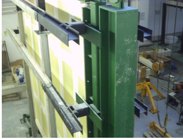
Figure 4. Lateral view on the rollers of the out-of-plane reaction system.
