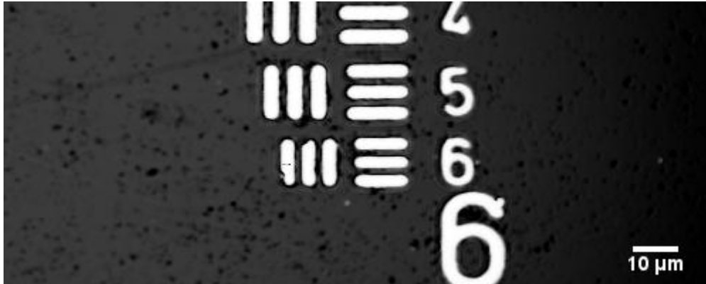
Figure 2. The transverse (X-Y) spatial resolution of the microscope is demonstrated with group 7 of Air Force Target, where parallel lines are 2.2\mu\text{m} apart.
