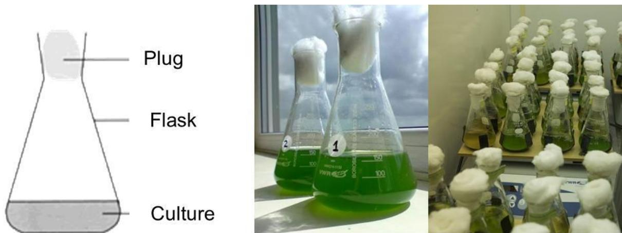
**Figure 4.1. Illustration of a flask culture, with single and multiple shaker arrangements.**
