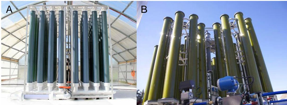
**Figure 6.11. Examples of vertically stacked column configurations.**
