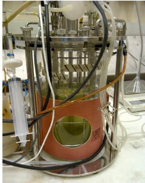
**Figure 4.2. Illustration and photograph of a miniaturised fermenter system.**
