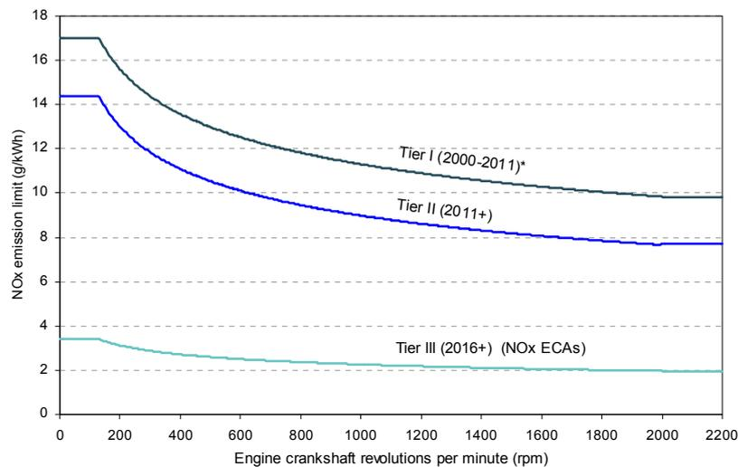
Figure 3: Default NOx limits as used in GloTraM
