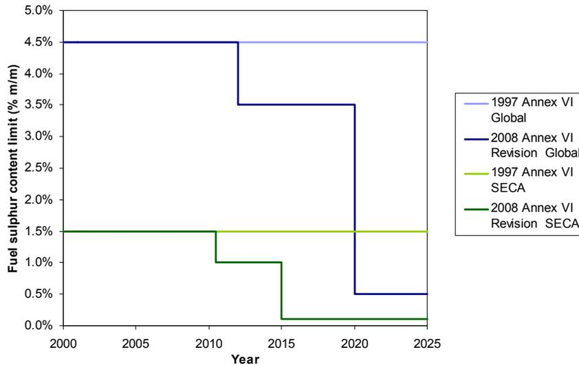
Figure 2: Default SOx limits as used in GloTraM
