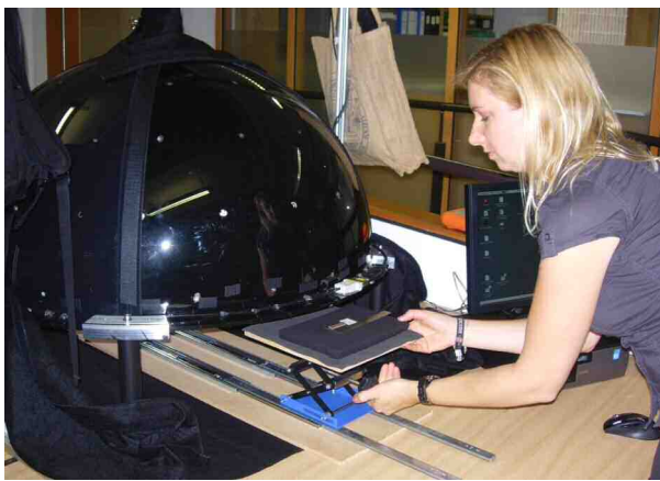
Fig. 2 Kathryn Piquette placing a leather sample into the RTI dome in the Centre for the Study of Ancient Documents (CSAD), Oxford University (Photo Susanna Harris).
