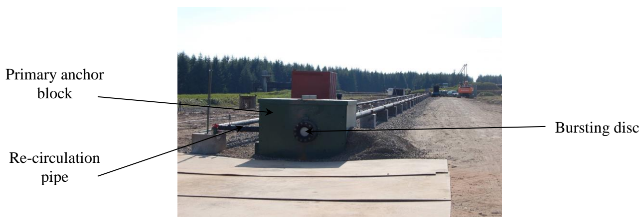
Figure 5.1: An image of the shock tube test rig from the rupture end, the primary anchor block and re-circulation pipe are visible in the left foreground.
