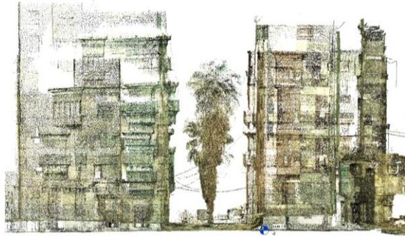
Figure 8. West Elevation from Laser Scanning
