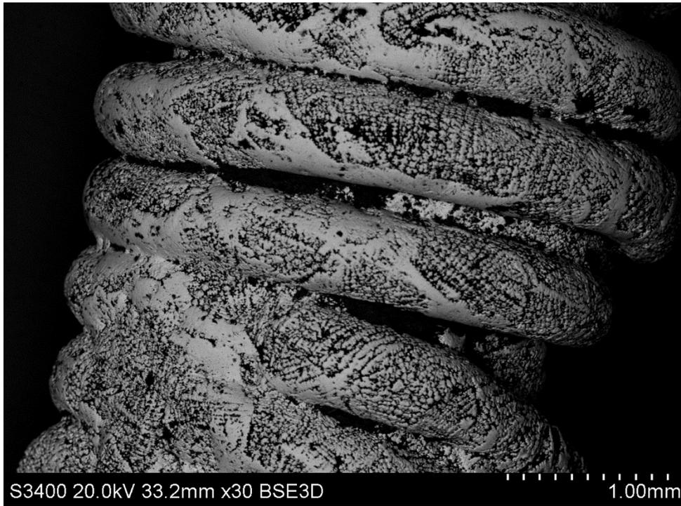
Figure 7. SEM detail of the headdress of *tunjo* O33895 from Tocancipá, showing the dendritic texture resulting from the slow cooling, as well as small filaments of metal connecting the thicker coils.
