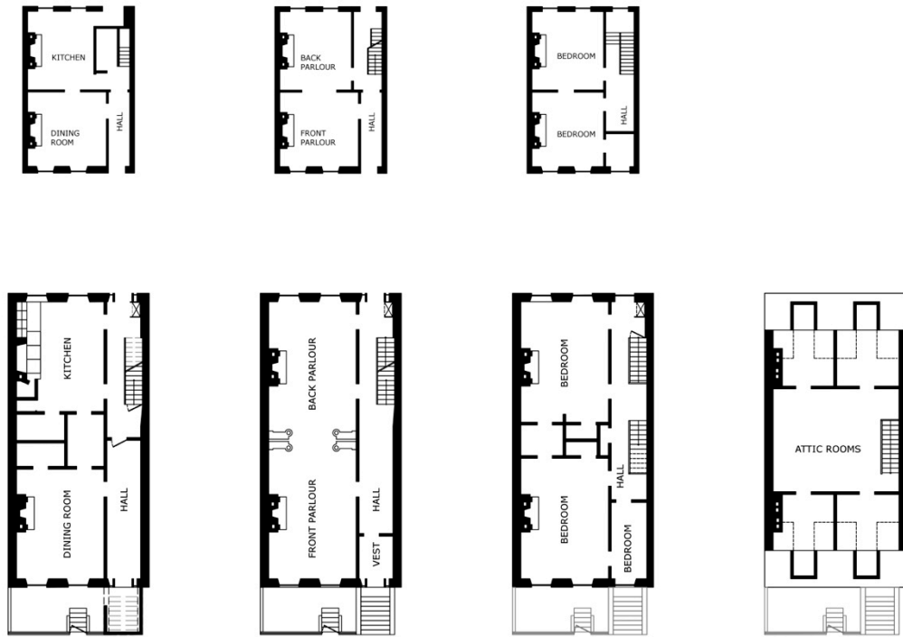
Figure 3. The row house: floor plans. Redrawn from Lockwood (1972, p.14-19) and Dolkart (2009, p.31).
