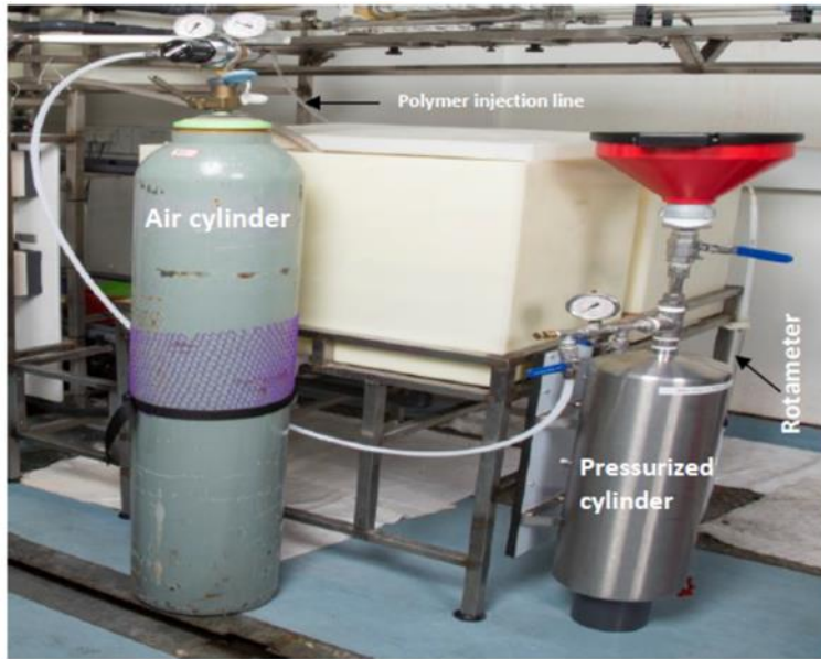
Figure 3-14 Photograph of pressurized polymer injection system
