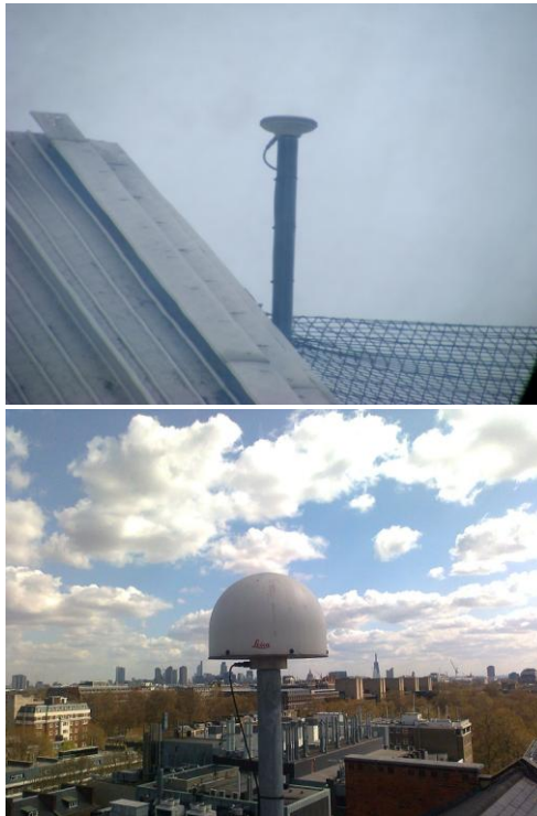
Fig. 1 Antennas of continuously operating GPS receivers at UEL (top) and UCL (bottom) that were used in the experiment. These stations are part of the Leica Geosystems 'SmartNet' real-time kinematic GPS network in the United Kingdom. Photograph used with permission from Leica Geosystems.
