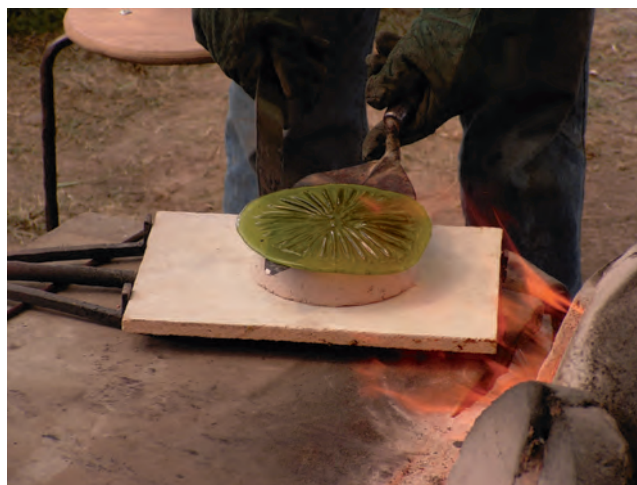
Fig. 6.3: Slumping of a glass disc over a bowl-shaped former. Replication by Mark Taylor and David Hill.
