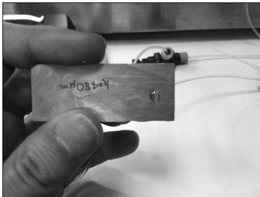
Figure 3.10 Photograph of the microseparator when it was leaking from the bottom of the silicon wafer with etching depth 480\mu\text{m} .
