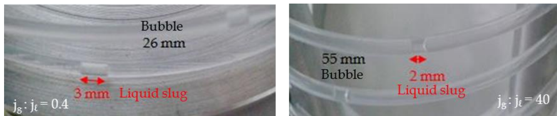
Figure 4.7 Observed flow pattern of the N 2 /methanol system at different gas-to-liquid ratios ( v_g=0.2\text{ml/min} , v_l=0.5\text{ml/min} on the left and v_g=0.2\text{ml/min} , v_l=0.005\text{ml/min} on the right) in a circular PFA capillary of 1mm inner diameter.
