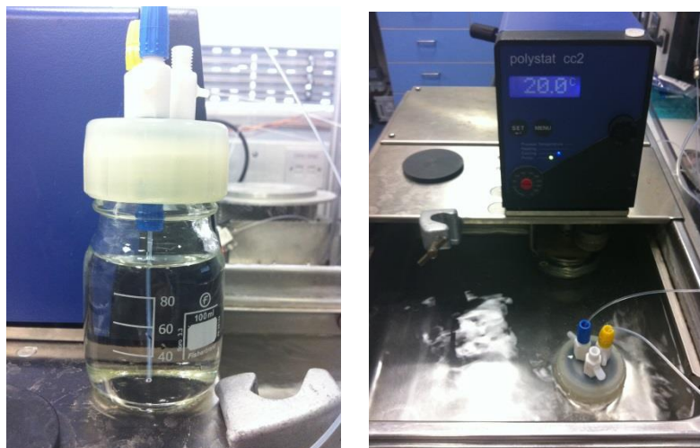
Figure A. 28 Photos of the set-up used for gc calibration of vapour MeOH. Bottle with MeOH bubbled with N 2 /He (on the left) and cooling bath used to maintain the temperature constant (on the right).
