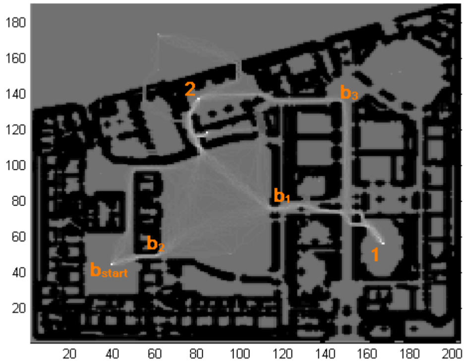
Fig. 46 The assignment clustering example with OC Map as background. The POAs go through the brighter cells more than the dark cells. Three key nodes b_1, b_2, b_3 are used to mark the clustering routes.
