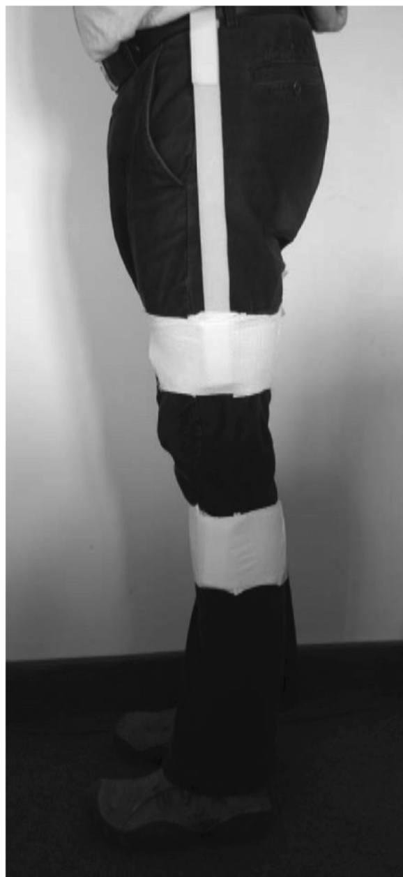
Figure 1 Positioning of the IMUs using Velcro straps on each thigh and shank. The straps could be applied outside clothing.
