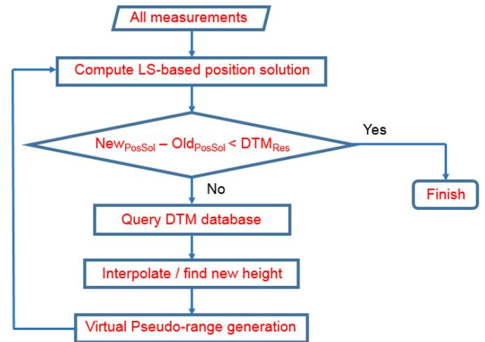
Figure 2. Terrain Height Aiding process
