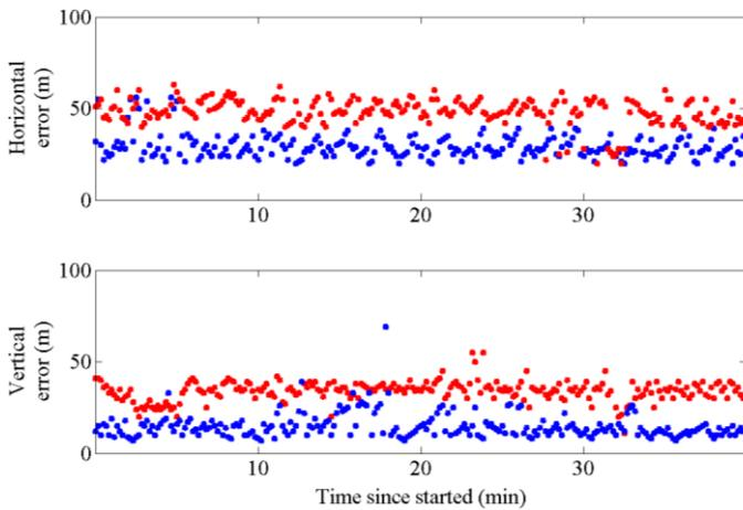
Figure 6. HORIZONTAL AND VERTICAL POSITIONING RMS ERRORS (ABSOLUTE VALUE) – TEST SET 1 (T3) FOR CASE WHERE NO HEIGHT AIDING IS APPLIED (RED) AND WHERE AUTOMATED HEIGHT AIDING IS INCORPORATED (BLUE) USING DTM 5 AND  $C/N_0$  WEIGHTING..
