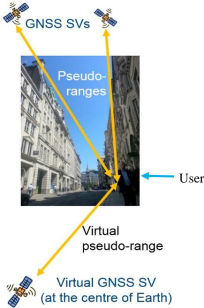
Figure 1. Terrain Height Aiding
