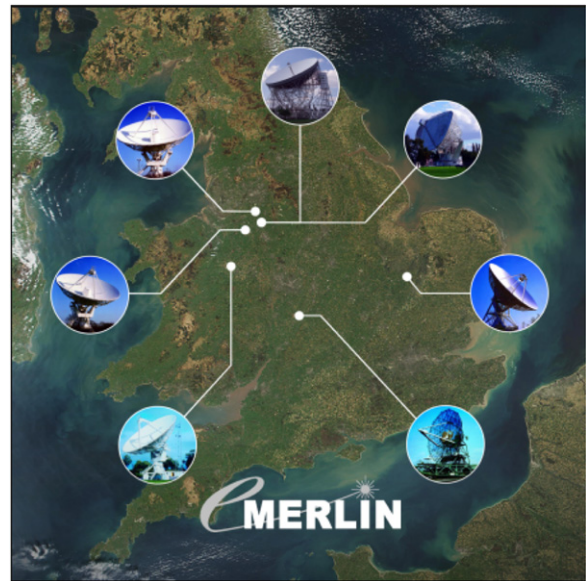
Fig. 2. Positions of the seven radio telescopes of e-MERLIN across the United Kingdom. Clockwise from top: Lovell, Mark II, Cambridge, Defford, Knockin, Darnhall and Pickmere. The longest baseline is 217 km, giving resolutions of 150, 40 and 12 mas at 1.3–1.8, 4–8 and 22–24 GHz respectively.
