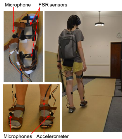
Figure 2. (left) Sandals with microphones, FSRs and accelerometer; (right) a participant during one condition 2 .
