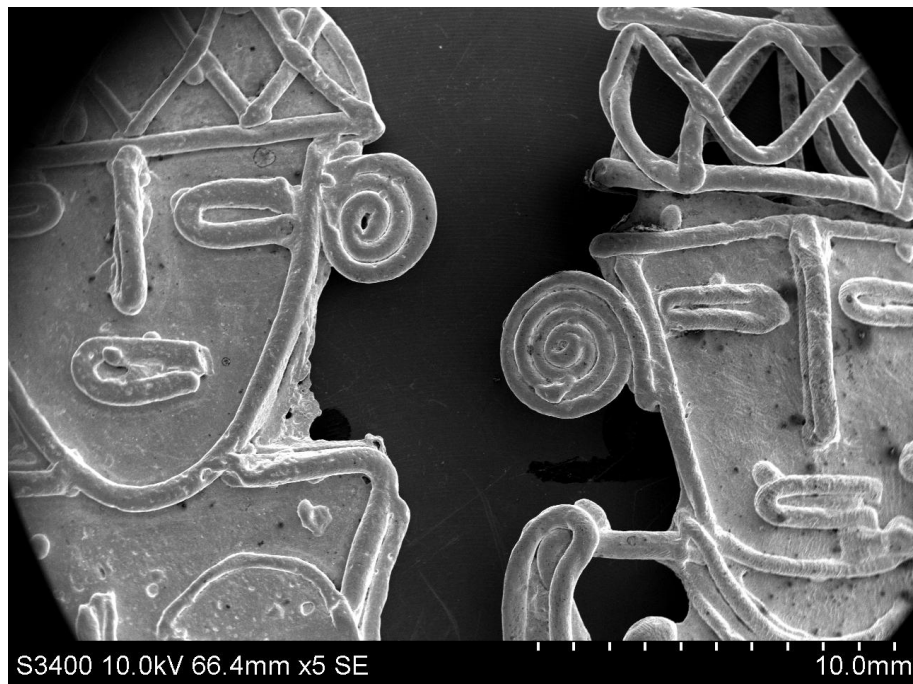
Figure 5. Scanning electron microscope image of two tunjos from Suba, showing detail of the waxwork on their faces and headdresses, including small balls of wax (now gold) used to stick together various wax parts before casting each figure in a single pour. A casting flash is visible at the neck of the figure on the left, while a casting void appears in the shoulder of the figure on the right.
