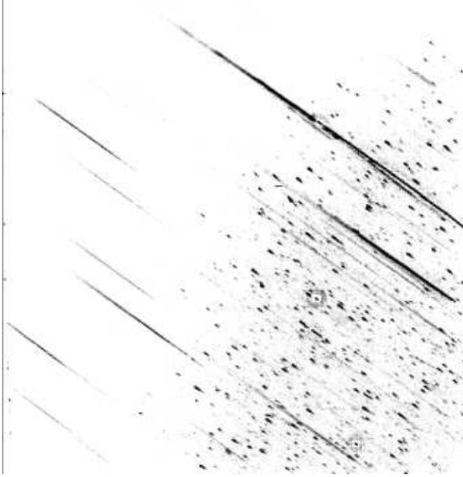
Figure 7. A typical detector image of the UV grism in clocked mode.
