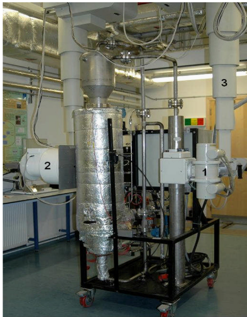
Fig. 1. Experimental set-up showing the x-ray equipment for visualizing the fluidized bed. (1) x-ray generator, (2) x-ray tube, (3) image intensifier.
