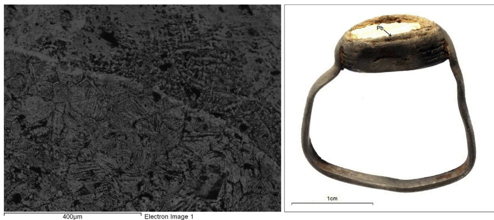
Fig. 5. a) SEM–SE image of the bezel soldering to the hoop of the signet ring. In the lower part of the image, the recrystallised microstructure can be observed on the surface of the ring while the dendritic structure of the soldering can be noticed in the upper area of the picture. b) Detail of the bezel formed by five silver strands, extensively worn. Note the burrs of the lead soldering over the white, powdery 'gem'.
