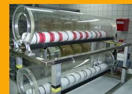
Figure 1 Rolling tank set-up
