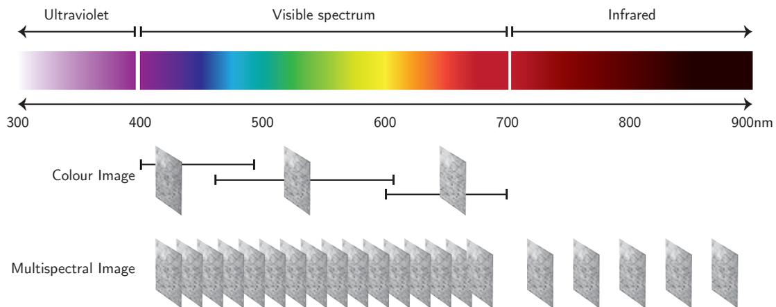
Fig. 2. Multispectral images are captured in a similar process as colour images. A colour image is a combination of three separate images captured at selected ranges of the visible spectrum representing blue, red and green tones. A multispectral image is captured as a combination of a series of images captured at discrete narrow ranges of the light spectrum.
