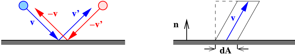
Figure 5.3: Illustration of boundary conditions in kinetic theory. (Left) Detailed balance: the blue scattering process \mathbf{v} \rightarrow \mathbf{v}' has the same probability as the red time reversed process -\mathbf{v}' \rightarrow \mathbf{v} . (Right) A particle emerging from a surface element dA with a velocity \mathbf{v} propagates into a skewed volume element dV = dA |\mathbf{n} \cdot \mathbf{v}| dt . This is the reason for the factor |\mathbf{n} \cdot \mathbf{v}| in the kinetic boundary conditions.
