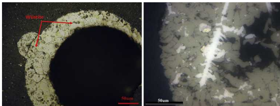
Fig. 13. Wüstite was occasionally identified within the matte prills (left). Dendritic iron particles (right).
