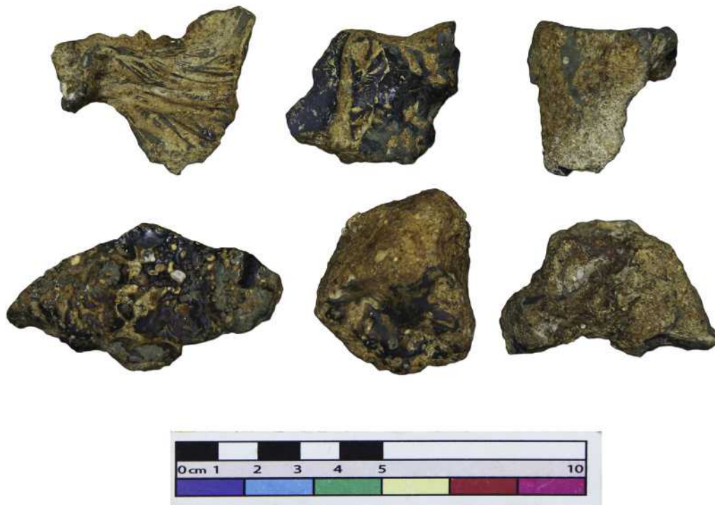
Fig. 5. Slag samples collected from the site of Baojia. Six fragments were selected from the Baojia slag samples, most of which look quite similar to each other. Flow pattern on their surface and sand inclusions on the underside indicate they were tapped from a furnace.
