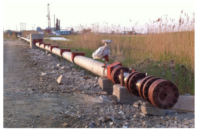
Fig. 1. Photograph of an instrumented 256 m long, 233 mm i.d. pipeline for experimental studies of CO 2 releases.
