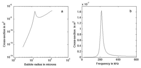
FIG. 1. Extinction cross sections: (a) variation in cross section with radius for 217 kHz, which is the resonant frequency for a 15- $\mu$ m bubble, and (b) variation with frequency for a single bubble with a radius of 15  $\mu$ m.
