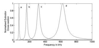
FIG. 3. The variation of extinction cross section with frequency for different bubble sizes, normalized to their maximum value. The bubble radii are (a) 50, (b) 20, (c) 10, and (d) 5  $\mu$ m.
