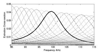
FIG. 2. A sample plot of the many individual cross sections that might add up to form the total attenuation. Most of the measured attenuation is due to bubbles that are not responding exactly at their resonance frequency, but resonate within approximately a bandwidth of the frequency of interest.
