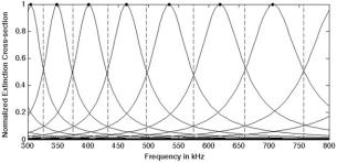
FIG. 4. A region of the spectrum showing the suggested frequency bin spacing and the cross section of the central bubble for each bin. Dotted vertical lines represent the frequency boundaries for the bins. The attenuation values used in the inversion will be at the frequency of the center of each bin (black filled circles), using interpolation between the measured acoustic data points.
