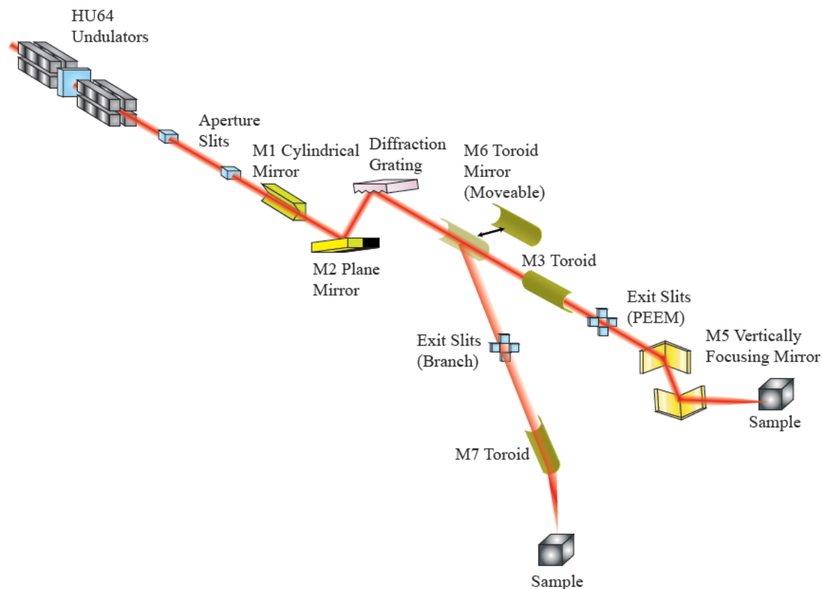
Fig 3.4: Schematic of main components of beamline I06 at the DLS [5].
