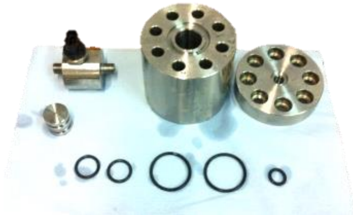
Figure 3.19: Dismantled fuel tank from pressure amplifier
