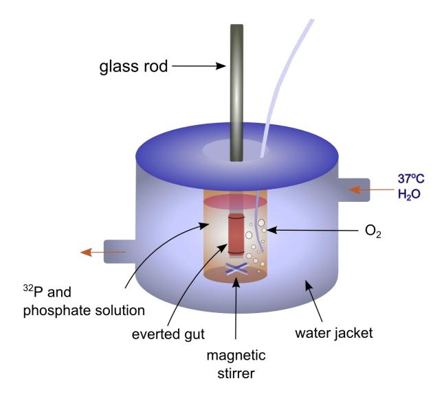
Figure 2.1. Diagram of in vitro everted sleeve technique method used for measuring Pi uptake
