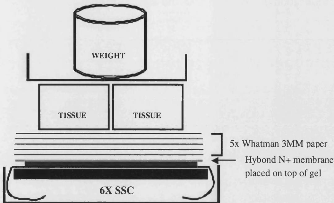
**Fig. 2.2: Illustration of set-up to blot DNA onto Hybond N+ membrane** (Amersham Pharmacia Biotech, UK) overnight.
