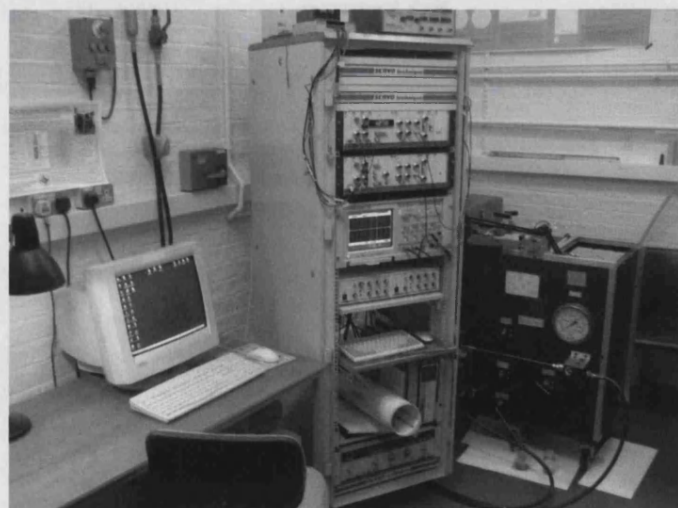
Figure 3-17 Hydrostatic pressure equipment housed in a temperature controlled laboratory. From left to right – data logging PC, electronics rack, and, most importantly, the servo-controlled measurement cell itself
