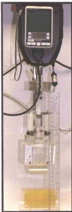
Figure 6.6 The Inspec 2200 mechanical testing device with attached ultrasound probe and load cell holder
