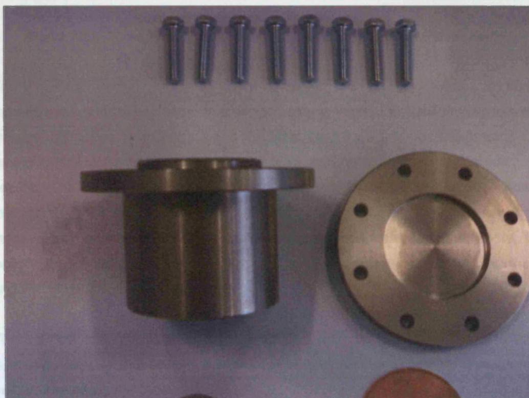
Figure 4.2.8: Photograph of design 3 showing the zinc bolts, nickel crucible and copper plate used in sealing (top) and a side view of design 3 showing protruding lip for sealing into the recessed lid (bottom).
