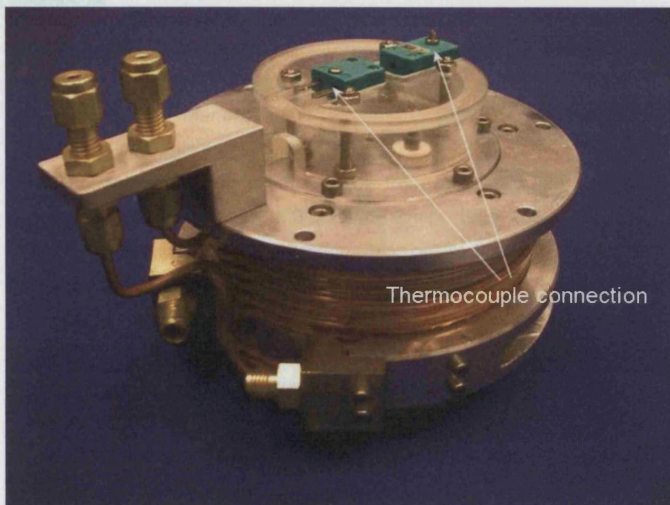
Figure 4.4.1: Side view of the custom built capillary furnace used at station 6.2 Daresbury.
