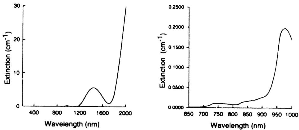
**Figure 8: The absorption spectrum of pure water**
