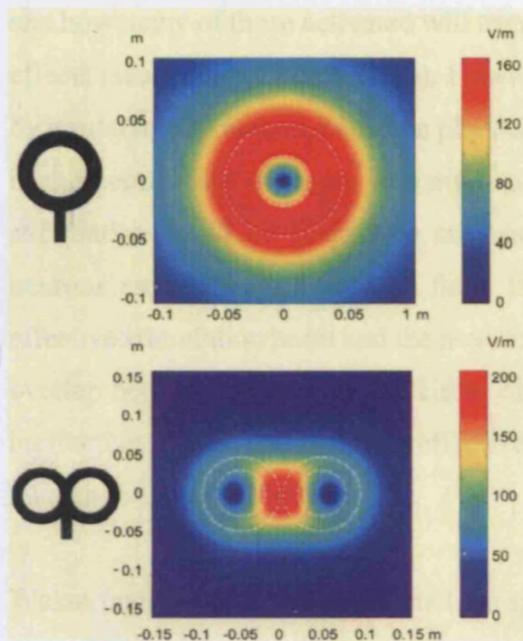
**Figure 4: Distribution of the induced electric fields by a circular (top) and figure-of-eight (bottom) stimulating coil.**
