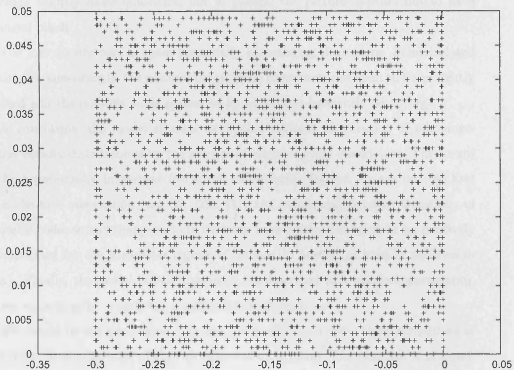
Figure 3.10: Computer generated image of low density flow. Each point represents the centre of a grain.
