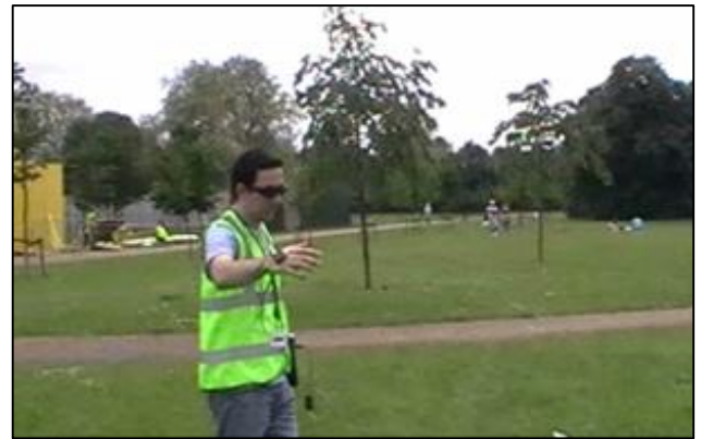
Figure 8. An example of using the Xsens MTi-G in a human MoCap experiment, with the antenna attached on the outside of the right hand and the IMU on the inside.
