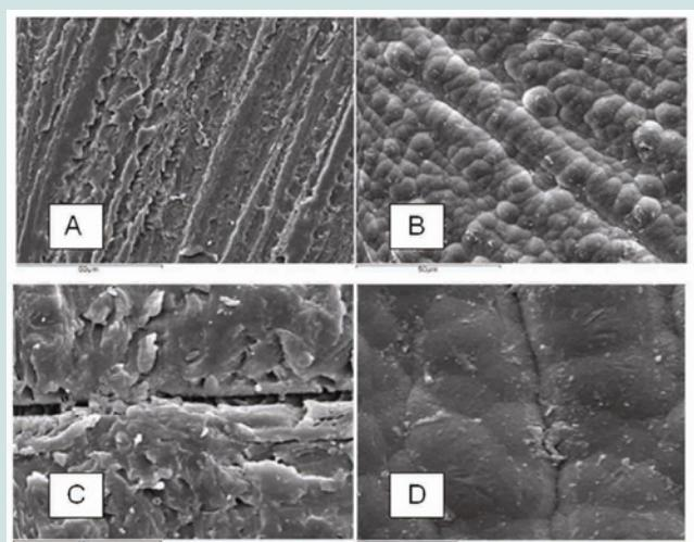
**Figure 3:** SEM images of uncoated (A and C) and a Parylene-coated (B and D) PMMA specimens at  $\times 1000$  and  $\times 3500$  magnification respectively.
