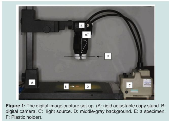
**Figure 1:** The digital image capture set-up. (A: rigid adjustable copy stand. B: digital camera. C: light source. D: middle-gray background. E: a specimen. F: Plastic holder).
