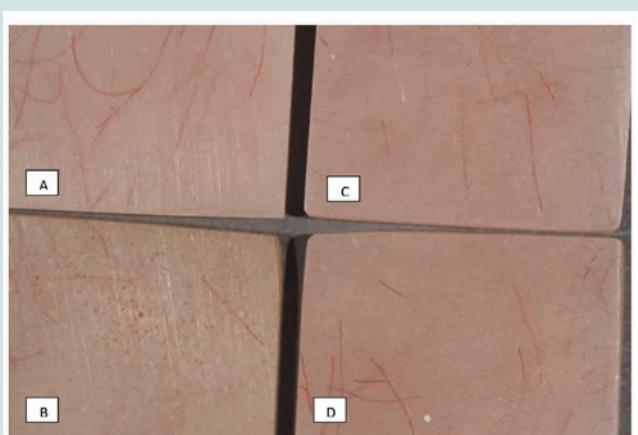
**Figure 2:** Digital image of different samples after one week immersion in the storage mediums: A) upper left: PMMA and water B) lower left: PMMA and coffee c)upper right: Parylene-coated PMMA and water d) lower right: Parylene-coated PMMA and coffee.
