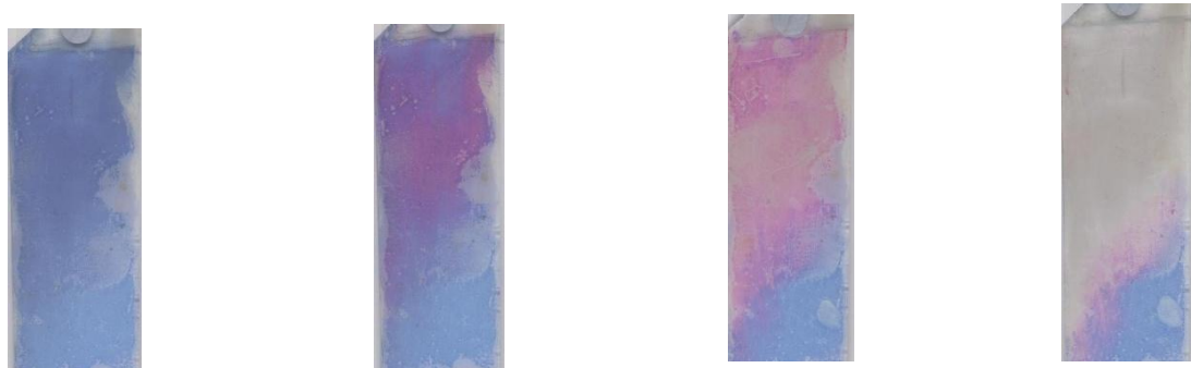
Figure 3.5(b) . Photographs of the changes in colour of resazurin intelligent ink sprayed onto a film of anatase/rutile (45x90 mm) formed at 500°C by AACVD on glass. The intelligent ink changes from blue → pink → colourless under irradiation with 365 nm light for 0, 1, 10, and 35 minutes.
