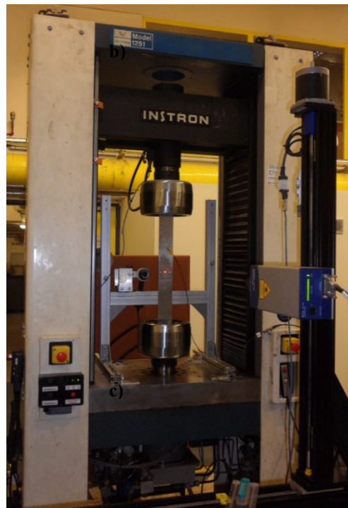
Fig. 1. Experimental setup: multi layer tensile specimen in fatigue testing machine with microscope for optical crack length measurement and laser interferometer.
