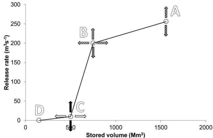
**Fig. 2.** Reservoir release rule (hedging) curves as represented by the IRAS-2010 model. Each patterned pair of opposing arrows represents an optimisation decision variable. Point D is the dead storage of the reservoir. Point A represents the controlled release when the reservoir is full. B and C points can be varied in two dimensions for hedging. In total 5 decision variables define each reservoir's release rule.
