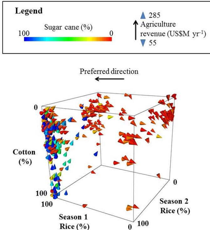
**Fig. 11.** 3-D (non-trade-off) plot showing the relationship between irrigation scheme selection and agricultural revenue. The solution points are the same as those shown in Fig. 10. High revenues can be achieved with or without the implementation of the cotton scheme. A high proportion of all other schemes must be implemented to achieve maximum revenue however.
