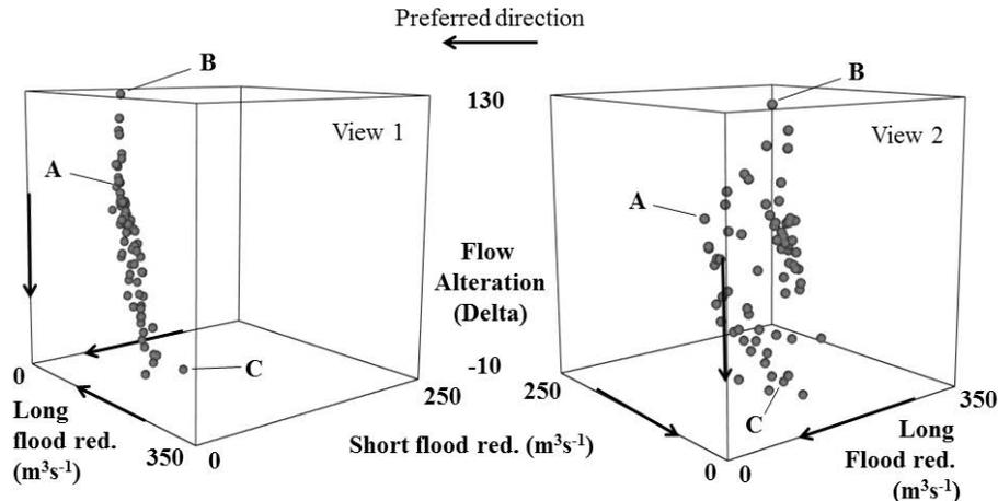
**Fig. 3.** Two views of the trade-off surface between flow related objectives. Flow regime alteration decreases as flood peaks are reduced allowing lower flows to be maintained closer to the natural regime. Three policies are highlighted and referred to in the text and subsequent figures. A 3-D animation of this plot is available in online Supplement.
