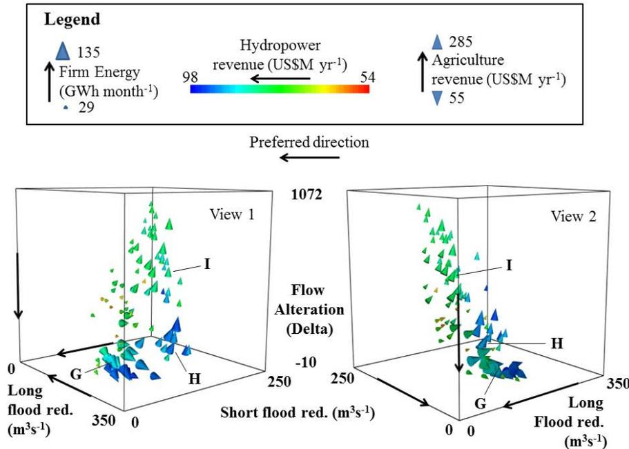
**Fig. 12.** The same trade-off surface as Fig. 10 but restricted to reservoir rules which result in no municipal deficits considering historical data. Such “brushing” of trade-off plots allow stakeholders to focus on system designs that interest them. Three policies are selected for discussion. A 3-D animation of this plot is available in online Supplement.
