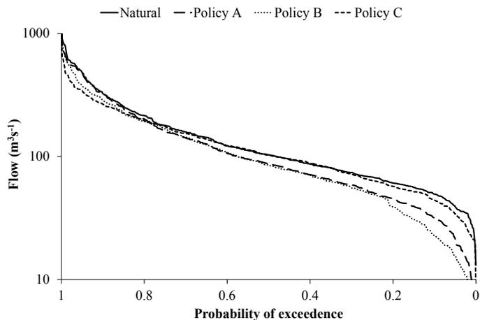
**Fig. 4.** Comparison of the flow duration curves resulting from Policies A, B and C of Fig. 3. Policy C allows around 20% of highest flows to diverge from the natural curve to augment lower flows, maintaining them closer to the natural regime. Policy A achieves the reverse.
