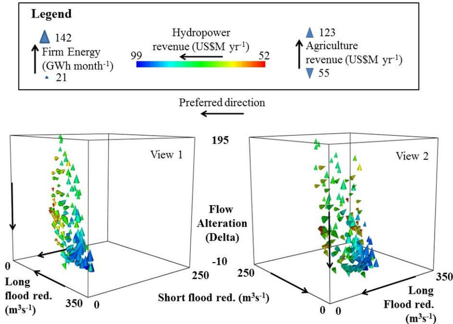
**Fig. 8.** The same trade-off surface as Fig. 5 with cones replacing spheres. Their orientation shows agriculture revenue from lowest (pointing down) to highest (pointing up). Agriculture revenues trade-off against flood peak objectives and correlate with firm energy, except at the highest agricultural revenues, where there is a trade-off.
