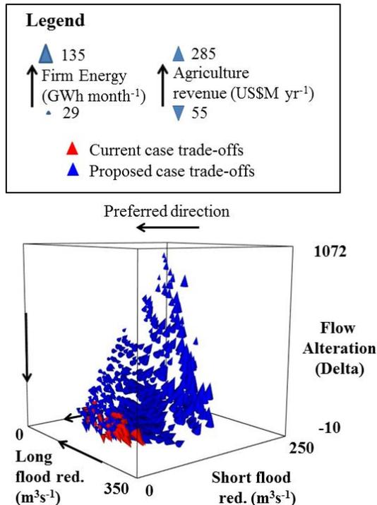
**Fig. 9.** Trade-off surface of the combined current and proposed demands cases (blue cones show system performance when irrigation schemes can be expanded). Some proposed demands solutions dominate the current demands solutions reducing their representation on the surface. This figure shows how trade-offs achievable by the best system operating rules change once irrigation investments are considered.
