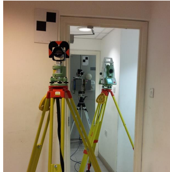
Figure 2 - Data Capture with Faro Photon (centre) with checkerboard targets and Leica TS15i (right)
